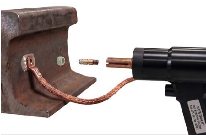
3. Prepare the materials and load the gun with the pin & ferrule.
