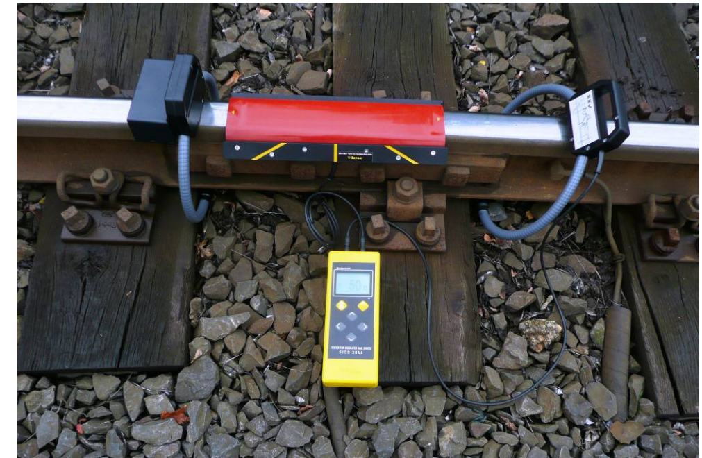
Fig. 3.4 C-sensor located before the next conductor branching off
