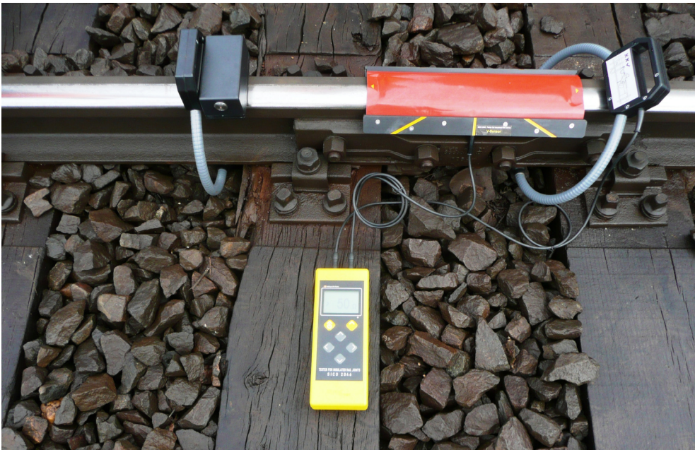
Fig. 3.8 C-sensor looped around rail and joint
