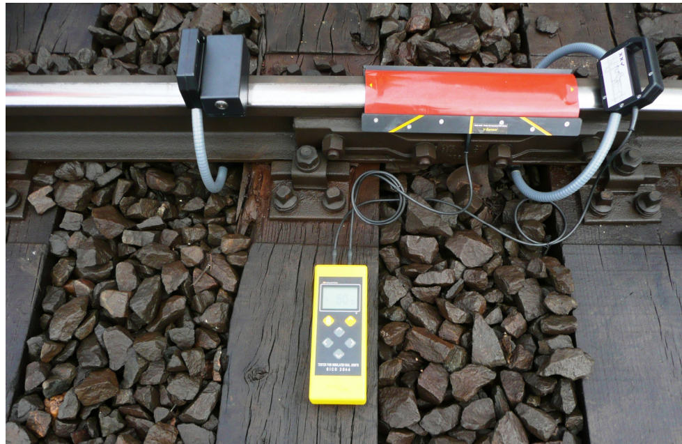
Fig. 3.6 C-sensor looped around rail and joint
